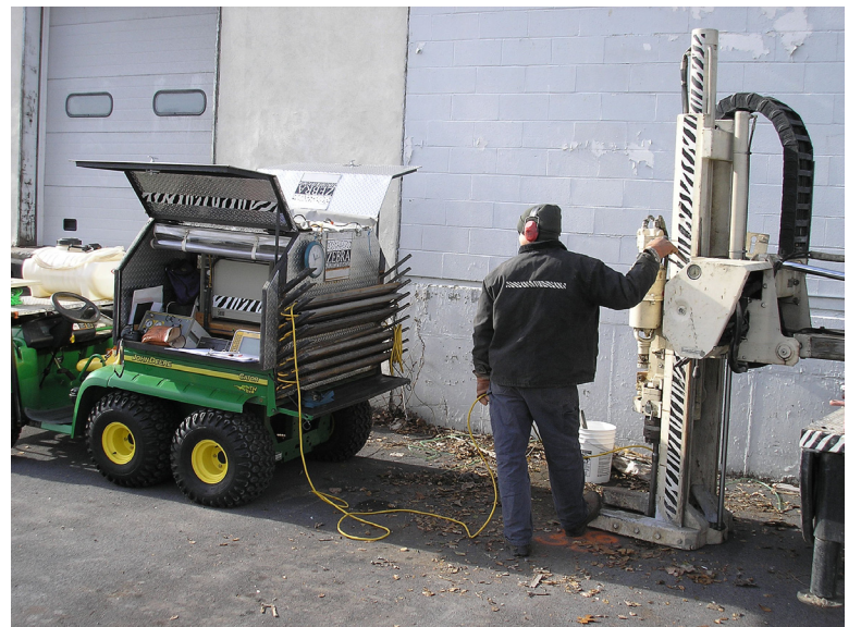
Ethan Plank, ZEBRA's Lead Probe Operator, pushes an MIP tool string with the 6620DT probe machine. The ZEBRA ATV-mounted MIP/EC unit (left) incorporates many of the latest system features from Geoprobe Systems® including trunk lines made of PEEK™ materials that minimize time required to clear the return line between logging locations, and the new MIP-Plus probes that operate at 110 VAC @ 5.5 amps.
